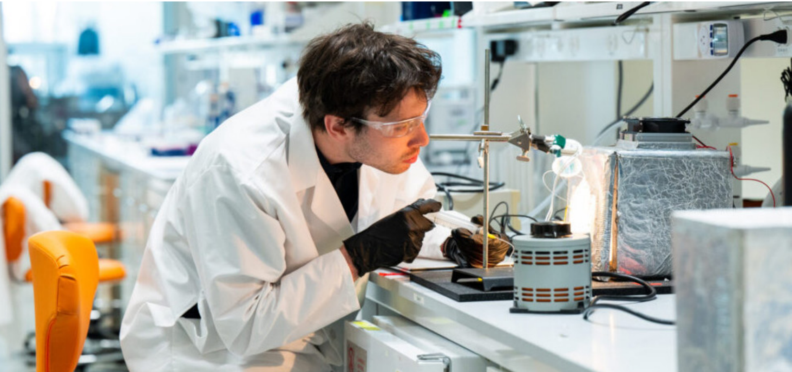
Doctoral candidate Raphael Kay MDes '22 tests the liquid window in a mock-house experiment to measure how much energy is needed for heating and cooling—a project supported by the Seed Grant Program and led by Joanna Aizenberg.
